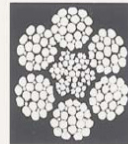
Internal corrosion whilst external surface shows little evidence of deterioration
