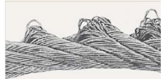
Looped wires as a result of torsional imbalance and/or shock loading
