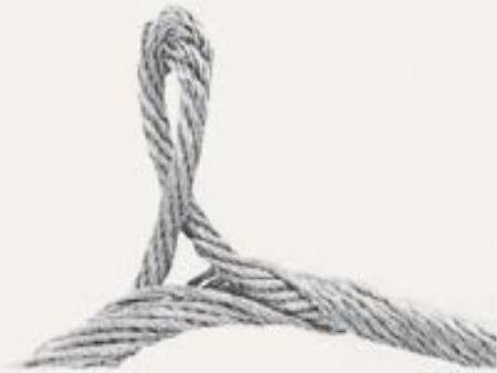
Protrusion of rope centre resulting from build-up of turn (‘core popping’)
