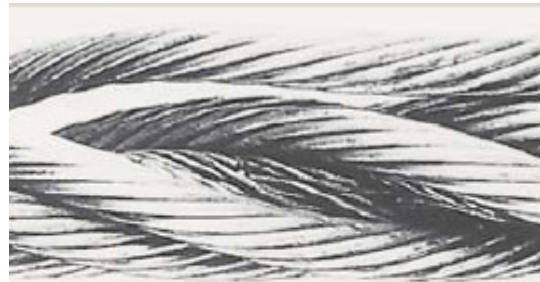
Break-up of IWRC, resulting from high stress application
