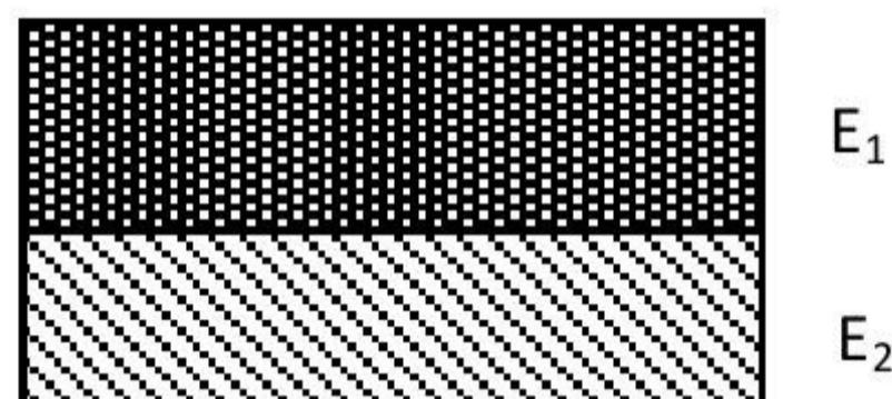
$$E_1 Q_1 + E_2 Q_2 = 0 \rightarrow E_1 Q_1 + \frac{E_2}{E_1} E_1 Q_2 = 0, \quad \frac{E_2}{E_1} = n_2$$
